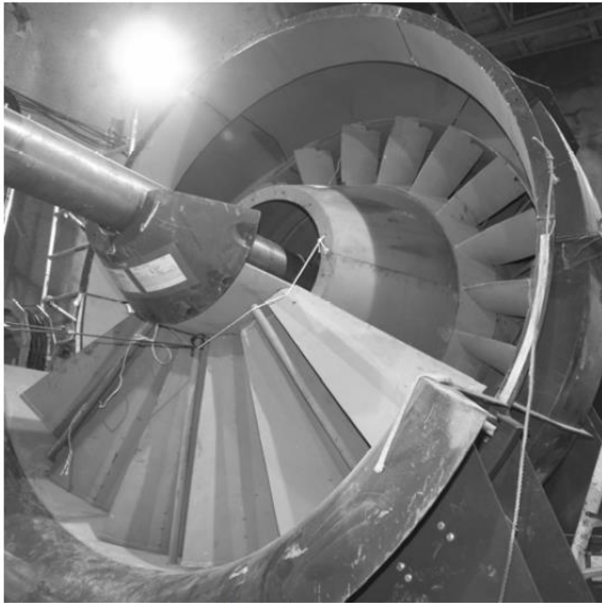
Figure 10. Mixed-flow fan under-construction, with impeller and Radial Vane Control evident.
