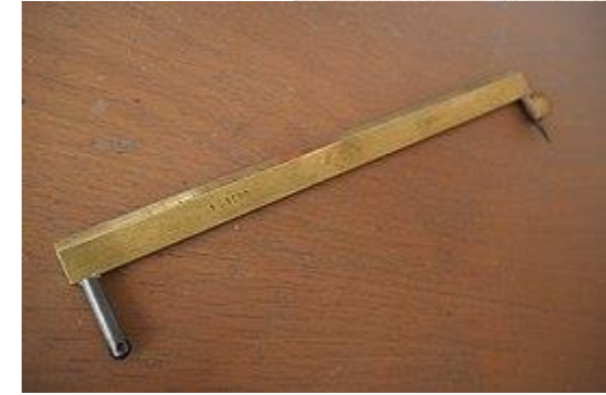
Prytz planimeter with wheel at the left
